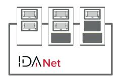
Through IDANet network-connection technology, Previdia Ultra control panels can be connected in a ring via a CAT5 ethernet cable (up to 100m) or optical fiber (by means of an appropriate SFP module according to the type of fiber used).
