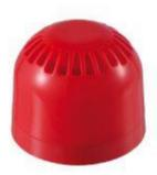
Inim ES0010RE addressable loop-powered sounder unit in red enclosure. Connects directly to the loop. Weatherproof to IP67, suitable for outdoor installation. Up to 106 dBA (adjustable), 32 selectable tones, 9...60 Vdc, 4-41mA (depending on tone).
