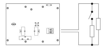
End of line resistor (R $_{\rm eol}$ ) = 5.6K $\Omega$ Alarm resistor (R $_{\rm w}$ ) = 2.2K $\Omega$
