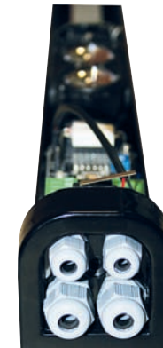
NEW ENCLOSURE WITH CABLE GLANDS
