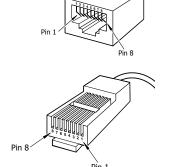
All the connectors must be shielded RJ45 type
